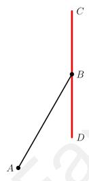
Arm  $\overline{AB}$  pivots back and forth around point A, sweeping out an arc of 60°, symmetric about the vertical line through A. The wiper blade  $\overline{CD}$  is attached to B at its midpoint and stays vertical as the arm moves. The arm is 3 feet long, and the wiper blade is 3.5 feet tall. What is the area of the windshield cleaned by the wiper, in square feet, to the nearest hundredth? (Assume that the windshield is a flat vertical surface.)
